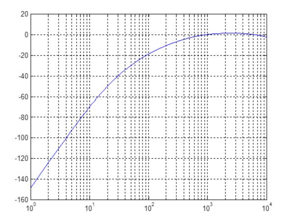
Figure 4.6: A-weighting values for Audio and Infrasonic Bands. Applying these weights will reduce the PSL at frequencies below 1 kHz. For example the measured PSL at 100 Hz will be reduced by 20 dB.
