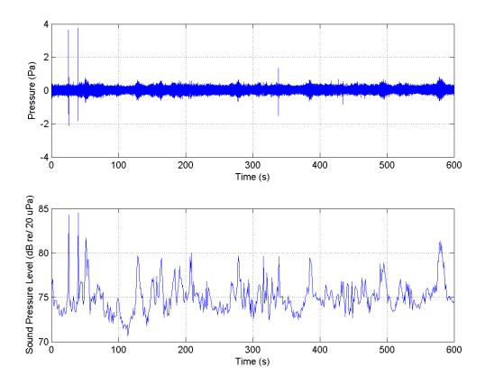
Figure A.50: Infrasound Data Recordings at New England Inst. of Technology 25 JUN 2013. (Channel 1 Time Series).
