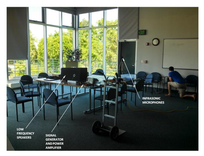
Figure 2.1: Calibration Setup 1.
