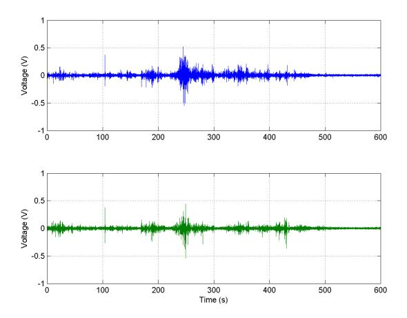
Figure 4.3: Voltage time series recorded by the two co-located infrasonic microphones. The two recordings are correlated in time and the voltage time series will be converted to a pressure time series using the receive sensitivity for each microphone.
