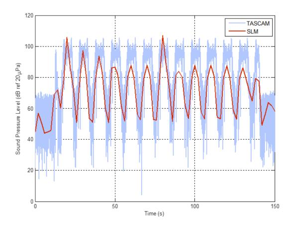
Figure 2.5: Comparison of SPL measurements computed from TASCAM with SPL measurements logged by SLM.
