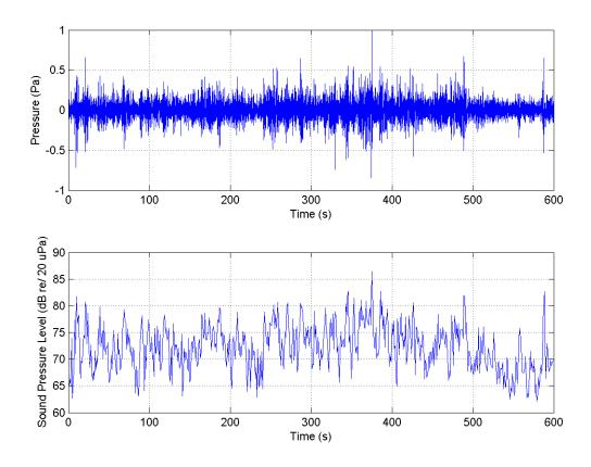
Figure A.28: Infrasound Data Recordings at Hodges Badge Co. 15 OCT 2013 at location 41 33 58.7 N, 071 15 22.5 W. (Channel 2 Time Series).
