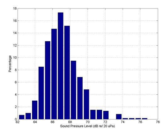
Figure A.57: Infrasound Data Recordings at Second Beach 08 OCT 2013. (Channel 1 Histogram).
