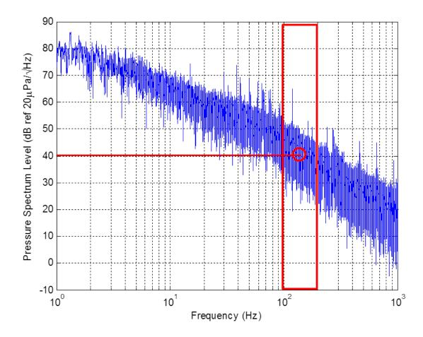
Figure 4.8: Example conversion of PSL to SPL. The example shown highlights the 100-200 Hz band. For this band the average PSL is approximately 40 dB and the corresponding SPL is 60 dB. If the entire un-weighted band were used, the SPL would be 80 dB.
