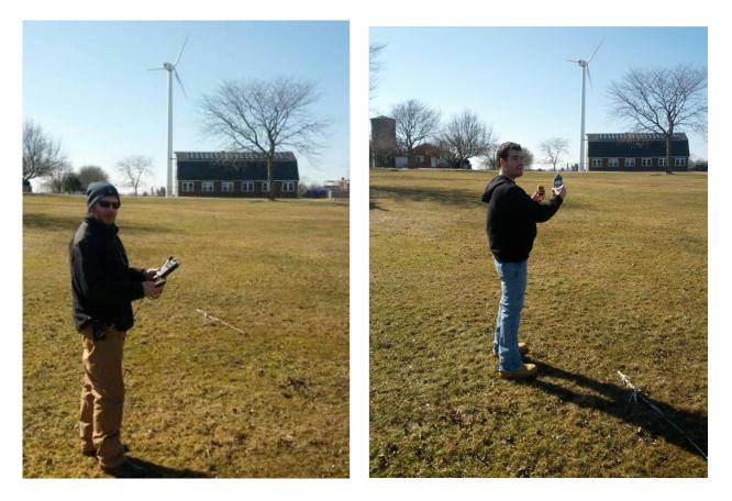
Figure 3.2: Data collection at Fisherman's Memorial Campground (RI-DEM). Left is the condenser microphone and audio recorder. Right is the SLM and GPS. Both must be time synchronized and merged post-test to generate geo-referenced measurements.
