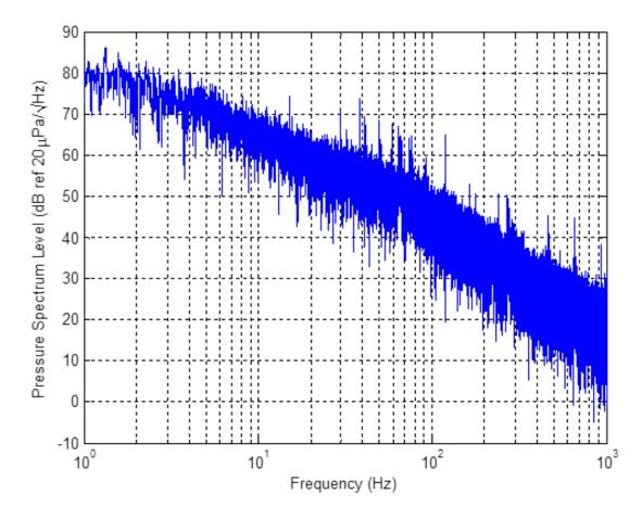
Figure 4.5: The voltage time series (converted to pressure time series using each microphone sensitivity) yields the un-weighted Pressure Spectrum Level. This representation shows the distribution of acoustic power as a function of frequency. Most of the acoustic power is concentrated in the low frequency (20 -200 Hz) and infrasonic frequency (1-20 Hz) bands.
