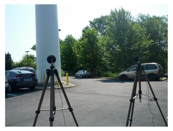
Figure 4.1: Infrasonic microphones for recording low frequency and infrasound for conversion to un-weighted SPL and PSL values. This photograph was taken at the New England Tech turbine location. The same instrument configuration was used at all sites.
