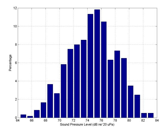
Figure A.29: Infrasound Data Recordings at Hodges Badge Co. 15 OCT 2013 at location 41 34 0.88 N, 71 15 17.24 W. (Channel 1 Histogram).
