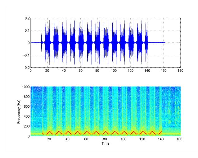
Figure 2.4: Voltage Time Series and Spectrogram for TASCAM recording system for LFM calibration signals.
