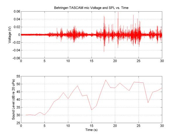
Figure 3.1: Example of TASCAM voltage time series and corresponding SPL.
