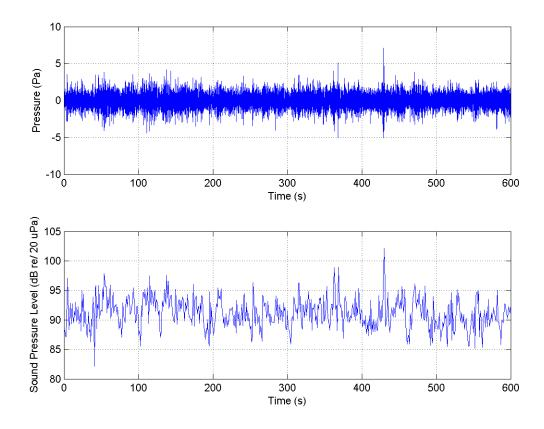
Figure A.56: Infrasound Data Recordings at Second Beach 07 OCT 2013. (Channel 2 Time Series).
