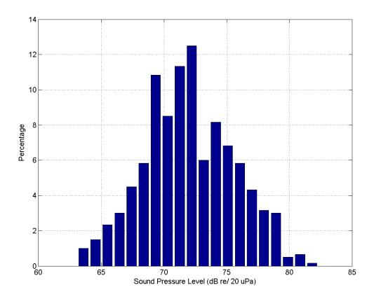
Figure A.31: Infrasound Data Recordings at Hodges Badge Co. 15 OCT 2013 at location 41 34 0.88 N, 71 15 17.24 W. (Channel 2 Histogram).
