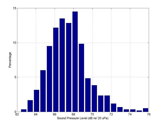
Figure A.59: Infrasound Data Recordings at Second Beach 08 OCT 2013. (Channel 2 Histogram).
