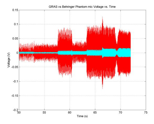
Figure 2.6: Comparison of Voltage Time series between Infrasound system and TAS-CAM system. The TASCAM and Infrasound System have different sensitivities (how much voltage is output for the same sound pressure). Because of the this the blue signal and red signal have different amplitudes. But the ratio between them is in agreement based on these different sensitivities.
