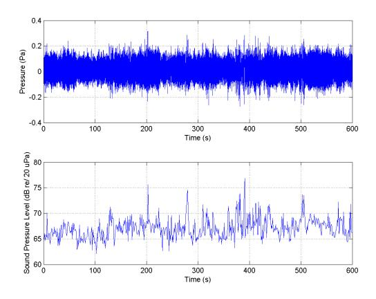
Figure A.58: Infrasound Data Recordings at Second Beach 08 OCT 2013. (Channel 1 Time Series).
