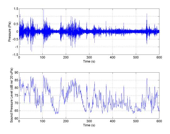
Figure A.24: Infrasound Data Recordings at Hodges Badge Co. 15 OCT 2013 at location 41 33 57.33 N, 71 15 17.18 W. (Channel 2 Time Series).
