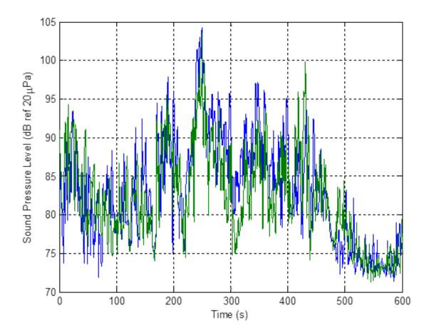
Figure 4.4: Sound Pressure Level values (un-weighted) computed from infrasonic microphone recordings. The levels are calculated from the RMS pressure over a one second window. As with the audio band recordings, these levels are consistently higher by approximately 18-20 dB, than the levels measured using the Sound Level Meter with A weighting.
