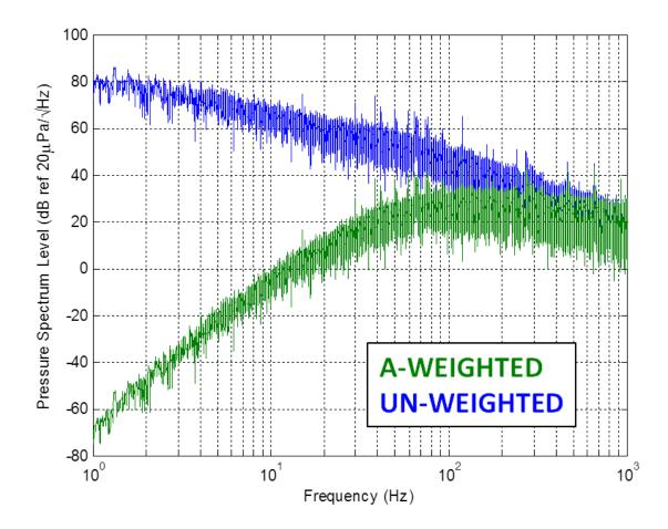
Figure 4.7: Comparison of Un-weighted and A-weighted PSL obtained from Infrasonic microphone. Because most of the acoustic power is concentrated at lower frequencies, a SLM that employs weighting will compute a lower SPL relative to an un-weighted measurement.
