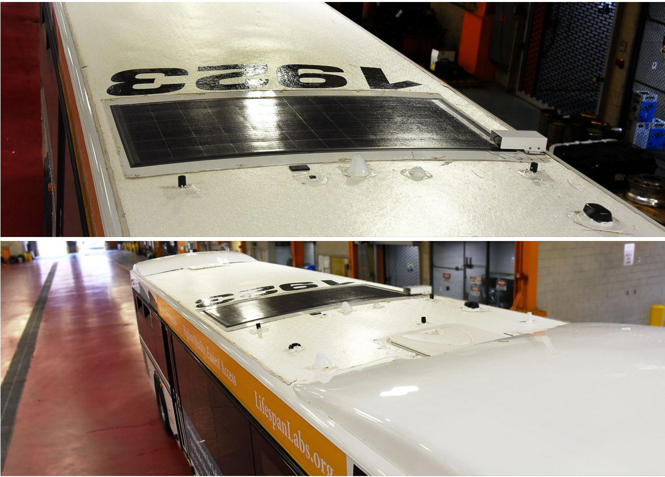
RIPTA installed auxiliary solar power system on diesel fleet
