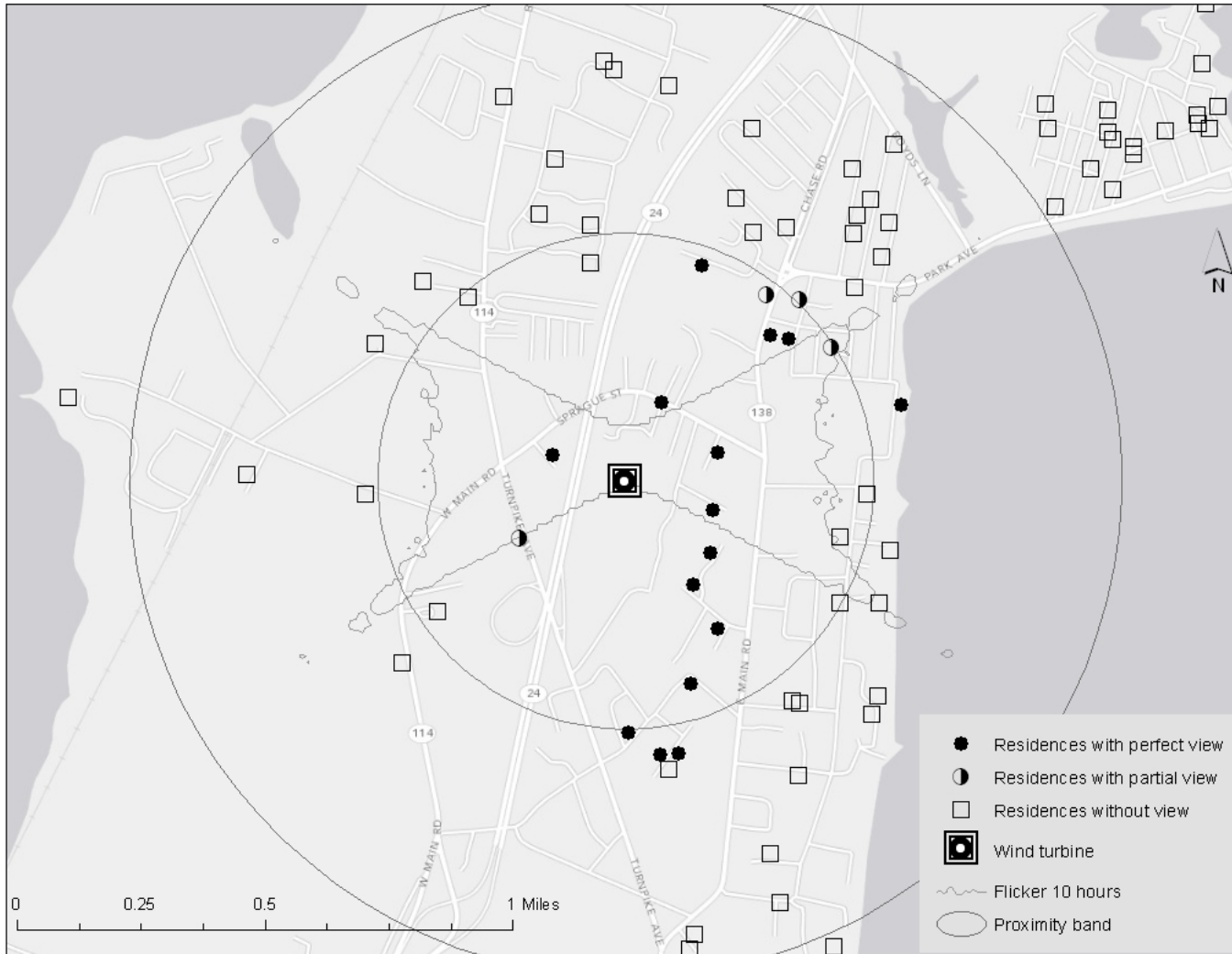
Figure 2: Proximity bands, viewshed, and shadow flicker, for post construction transactions around Portsmouth High School wind turbine
